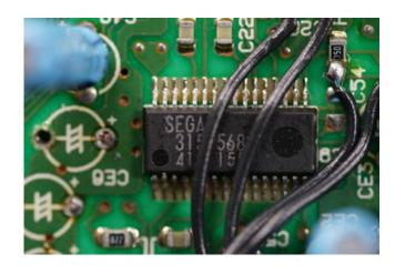
The main difference between the mainboard in this console and earlier revisions (excluding VA2 and VA2.3) is that the pair of quad op-amps in the audio amplifier on VA0, VA1 and VA1.8 boards is gone. In its place is a Sega 315-5684 chip, manufactured by ROHM. This is a
