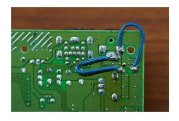
On the underside of the mainboard, Sega has installed two blue bodge wires. Not all boards in this revision have these wires, so it's difficult to say exactly why they are there. We speculate that Sega's engineers may have judged the traces on the mainboard to be
