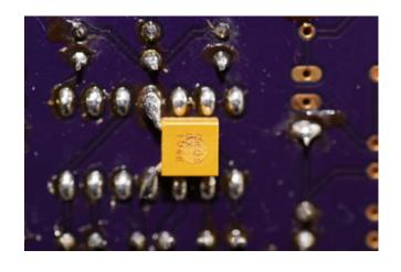
because there was no room in the upper footprint of the board for it, reflecting the preliminary state of this design. There also appears to be no power filtering on the Mega Amp for 5V.
