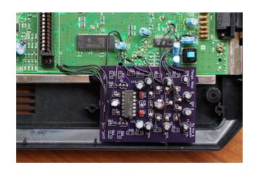
The Mega Amp in this console follows an unfiltered setup. This means that the cutoff frequency for the low-pass filter is 21.16 kHz, achieved by using 160 Kohm resistors and 47 pF capacitors on the amplifier (due to the extreme amount of inaudible high-frequency sound produced by the YM2612 and YM3438, a low-pass filter is necessary to prevent distortion).
