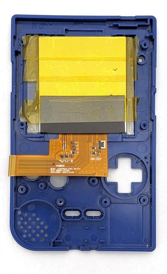
Set the LCD in place and insulate the back with Kapton tape to protect your screen from shorting—when modding, you want to avoid stacking conductive materials atop one another. Keep in mind that the screen is much smaller than the viewport and you will be able to see into the space around it. If you don't want to see the Kapton tape around the edges, cut it more precisely than we did!
