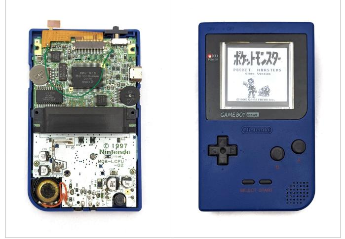
Screw the PCB to the board using the Philips Head screwdriver and then close the shell using the Tri-Wing screwdriver.
