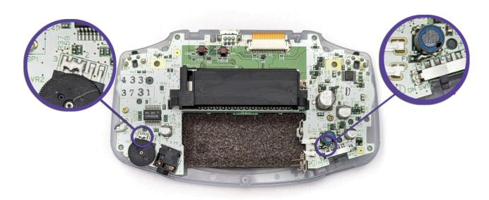
Since we're no longer using batteries, we can bypass the F1 fuse by bridging it to the inductor. Add a generous amount of
