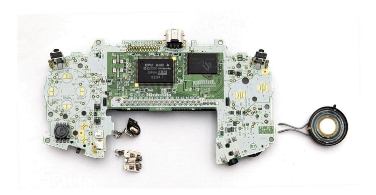
Remove the clock crystal from the mainboard. Depending on your board revision, it will either be black or silver. For the black version, touch a blade-tip soldering iron to the two soldering pads under the left side of the oscillator and gently flip it over. If you have the silver version, twist it off with a pair of pliers.
