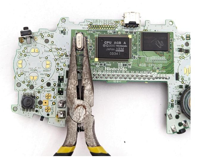
Finally, remove the battery contacts by heating the soldering pads while gently wiggling the contacts with a pair of needlenose pliers. When the solder melts, the contact will slide out. Do one at a time. If necessary, use a solder pump to remove excess solder to give you more room to work.
