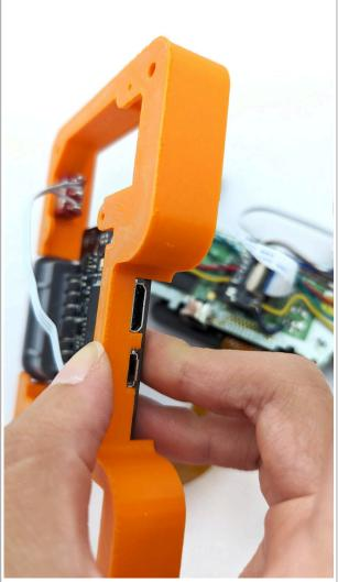
It's very important to make sure that the ribbon cables are feeding through the case at this point. If they're not, you'll have to remove the cables and reattach them to the GBA PCB in order to get it to fit in the case. If you do have to remove the ribbon cables to fit everything in, make sure you test your kit again!
