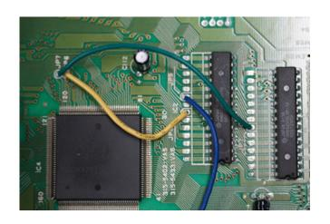
The top of the motherboard features several "bodge wires," soldered point-to-point in order to fix factory defects on the board surface (the alternative would be making an entirely new PCB). These wires carry "enable" signals, which Sega's custom chips generate,
