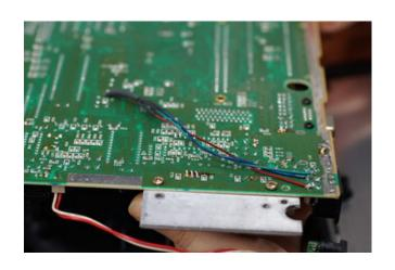
soldered and heat-shrunk connection in the middle of each of these wires.
