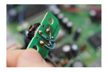
The audio connection for the Neobitz board has been tapped from the headphone out. Again, this is an older modding technique, which predates the recent practice of pulling audio from the pre-amp on the CXA1034 chip (Sony's headphone amp chip).
