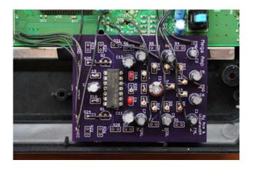
There are some visible bodge wires on the Mega Amp itself. It was originally designed with a transistor buffer on the stereo outputs in order to drive headphones for a Sega Genesis model 1 VA7. However, this didn't work all that well, and produced audible clipping.
