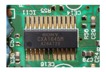
adjustable gain and low-pass filtering through external resistors and capacitors. On the Genesis model 2 revisions that use this configuration (VA2, VA2.3, VA3, VA4), it delivers audio from the internal preamp to the expansion connector for passthrough to the Sega CD model 2. The video encoder is also different; there can be up to 4 different chips in use (Ace has confirmed 3 of them). This particular console has a Sony CXA1645.
