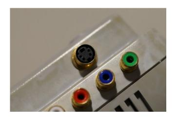
The addition of the ports is another matter. With the correct cables, the multi-out port on a Super Famicom or SNES can already output composite video, S-video and RGB. The latter is the best quality signal, but it is usually delivered through a SCART. This
