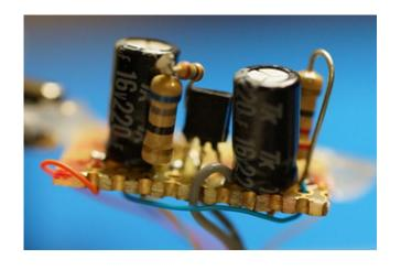
... then goes to a split where a 25 ohm and a 68 ohm resistor chained together (by the left capacitor) go to ground on one side.
