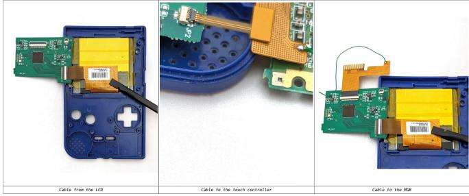
Note on the brightness controller: the MGB doesn't include a spot for the brightness controller. Brave modders can take a Dremel to the shell to create an access port to the brightness controller. Alternatively, you can skip connecting the touch controller cable altogether and use the screen at its standard
