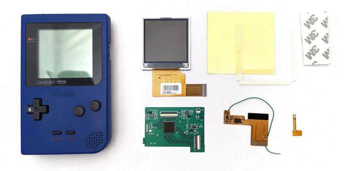
We used a kit sourced from Retro Modding, which included the backlit liquid crystal display (LCD), the printed circuit board (PCB) and attending ribbon cables, a piece of 3M foam tape, and a 3D printed bracket. According to the product description, the kit is supposed to include a three-piece laser cut bracket in place of that last item; the 3D printed bracket we received didn't fit the MGB shell, but we were able to improvise with the pieces we had on hand.
