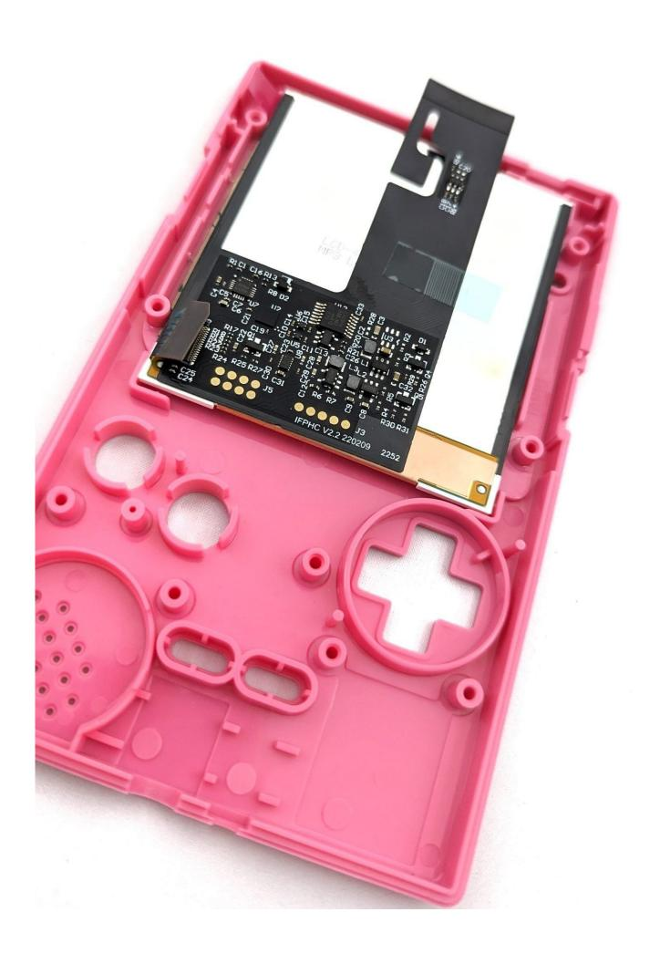
Use the double-sided adhesive included in the kit to fix the screen in place. Peel one layer of backing from the adhesive and stick it in the shell. Ensure that it's not bubbling (you can use the spudger again to do so). Then, peel the backing from the other side of the tape.
