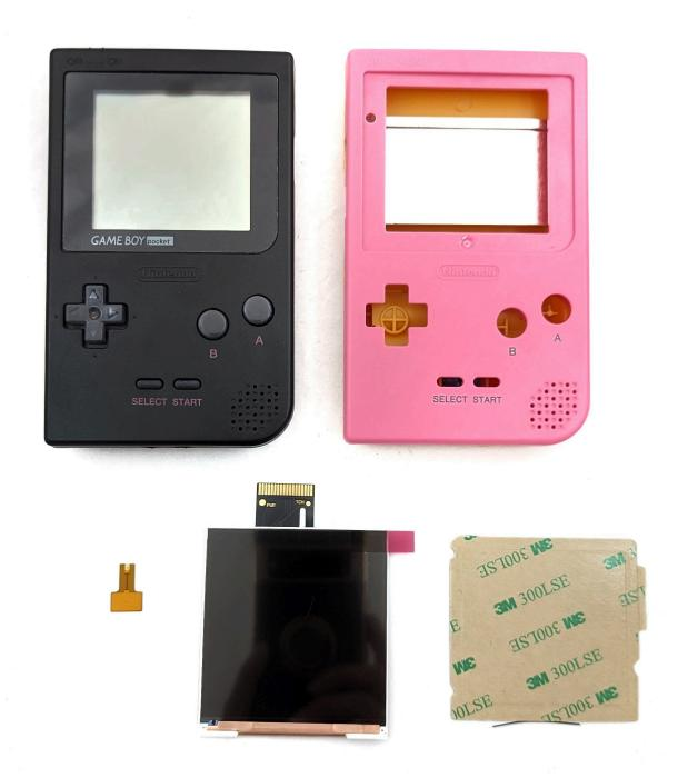
This kit is sourced from FunnyPlaying and includes the IPS LCD with its attending ribbon cable, an adhesive gasket, and an optional touchpad to solder to the ribbon cable.
