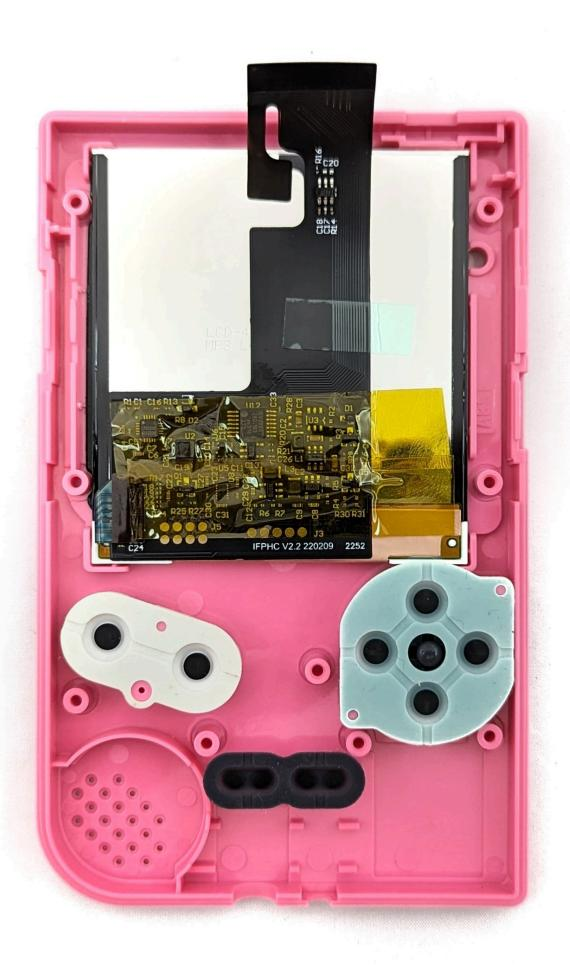
When working with electronics, you want to avoid stacking conductive materials on top of one another in order to avoid shorting. To that end, we recommend insulating the LCD with a layer of Kapton tape before connecting the Game Boy Pocket PCB.
