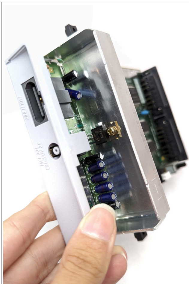
One screw, holding the heat shield in place
