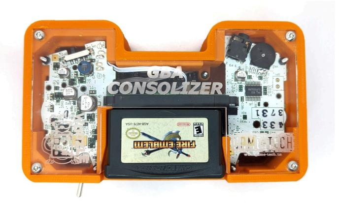
Feed the four remaining screws through the holes and fix them in place using the nuts. Try not to exert too much force against the plexiglass when you screw them in.
