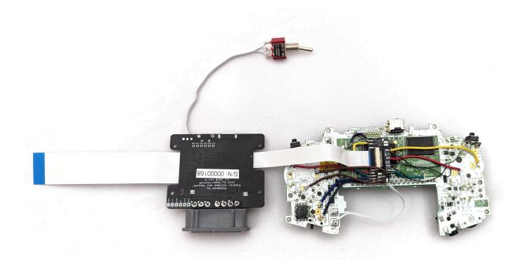
Note: there are two major versions of the GBA, a 40-pin version (identified with serial numbers beginning with a 0) and a 32-pin version (identified with serial numbers beginning with a 1). The kit only includes a ribbon cable for the 40-pin version. The easiest option is to mod a 40-pin GBA. If, however, you only have a 32-pin system, then you will have to order a separate cable to complete the mod.
