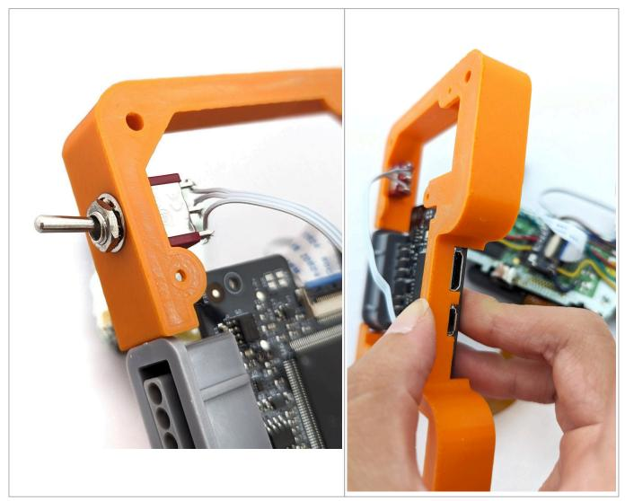
It's very important to make sure that the ribbon cables are feeding through the case at this point. If they're not, you'll have to remove the cables and reattach them to the GBA PCB in order to get it to fit in the case. If you do have to remove the ribbon cables to fit everything in, make sure you test your kit again!
