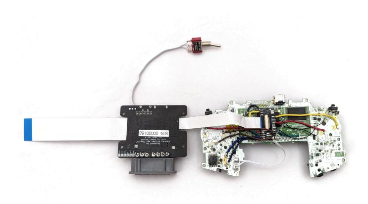
**Note:** there are two major versions of the GBA, a 40-pin version (identified with serial numbers beginning with a 0) and a 32-pin version (identified with serial numbers beginning with a 1). The kit only includes a ribbon cable for the 40-pin version. The easiest option is to mod a 40-pin GBA. If, however, you only have a 32-pin system, then you will have to order a separate cable to complete the mod.
