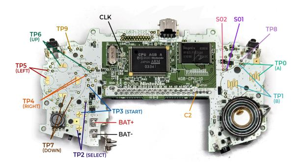
In both cases, don't forget to solder the battery terminals! The kit includes 3 inches of 28 awg 2 conductor ribbon cable for the power (BT+) and the ground (BT-), the positive and negative battery terminals. Make sure that you don't switch these or the kit won't work!
